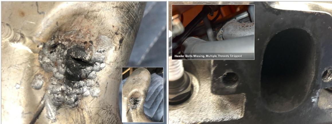
▲ Header Damage – Exhaust Leaks
