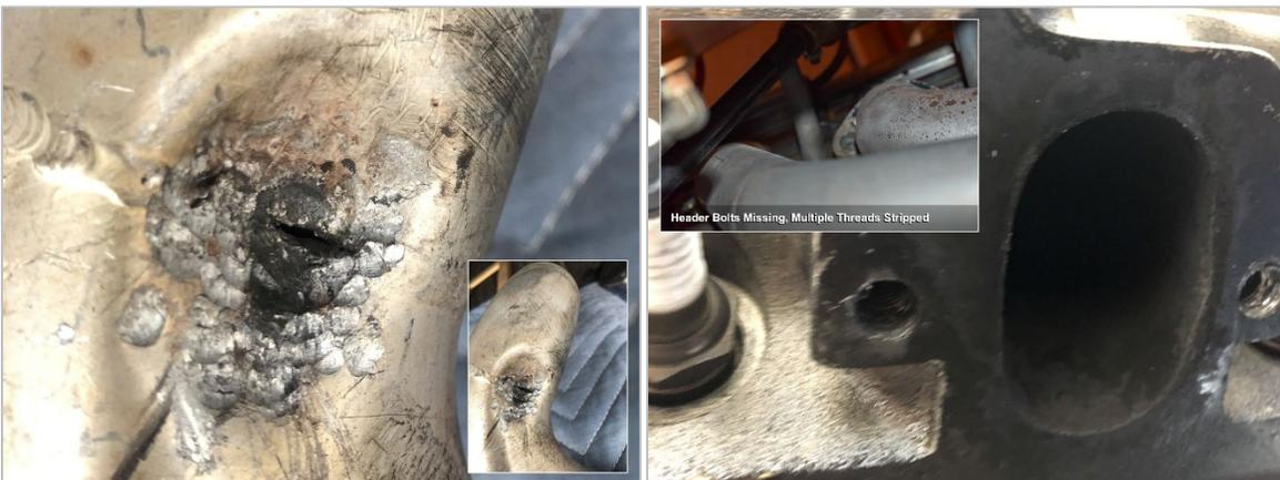
▲ Header Damage – Exhaust Leaks
