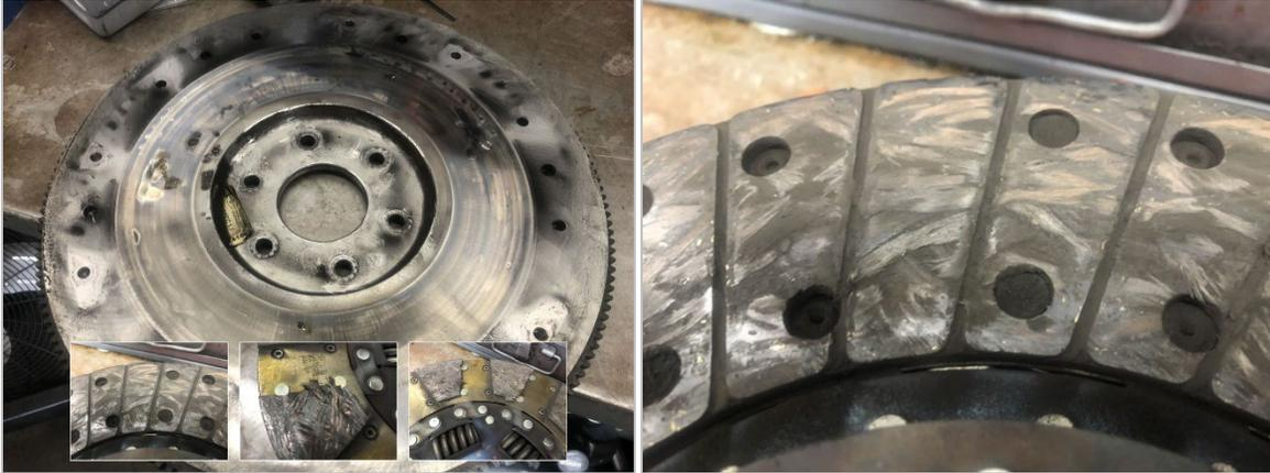
▲ Flywheel and Clutch Damage
