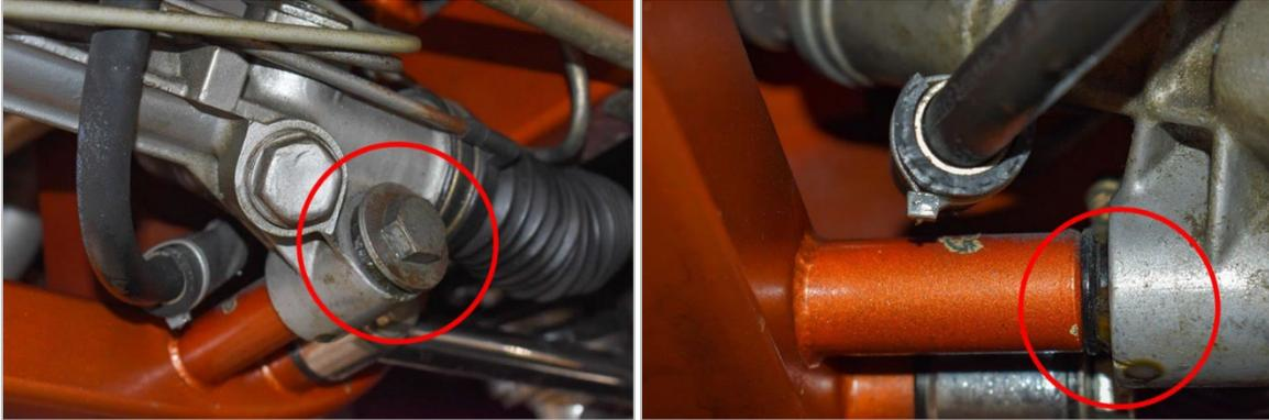
▲ Fluid Leaking from Rack and Pinion
