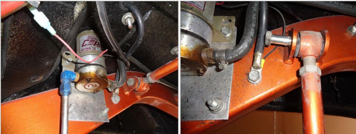
▲ Fuel Pump Leaking – Control Arm Bushing Damage
