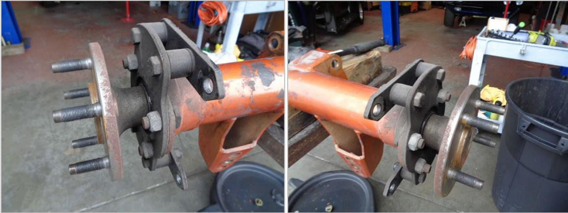
▲ Disassembled Rear End Axles
