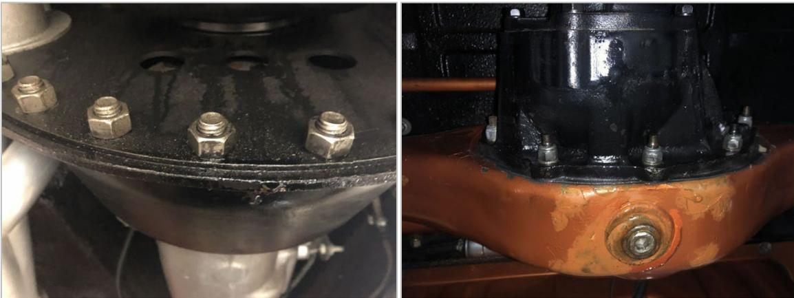
▲ Rear Engine Seal Fluid Leak – Third Member (Rear End) Fluid Leak
