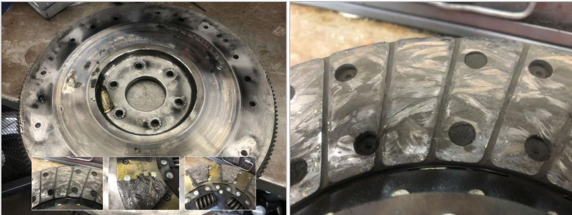
▲ Flywheel and Clutch Damage
