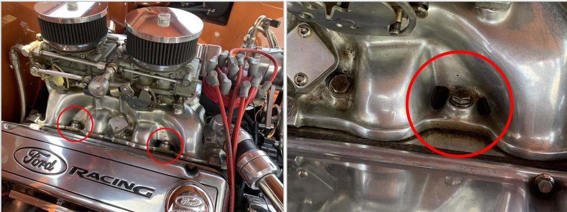
▲ Oil Leaking from Around Manifold Bolts
