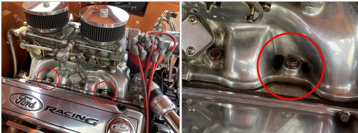
▲ Oil Leaking from Around Manifold Bolts
