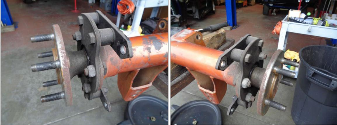
▲ Disassembled Rear End Axles
