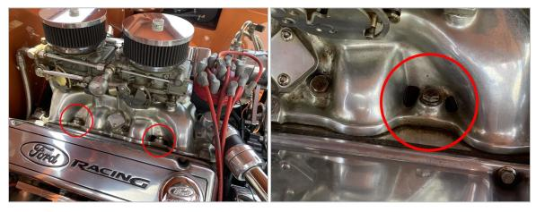
▲ Oil Leaking from Around Manifold Bolts
