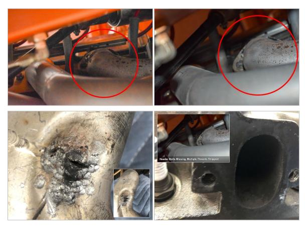
▲ Header Damage – Exhaust Leaks
