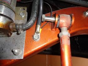
▲ Fuel Pump Leaking – Control Arm Bushing Damage
