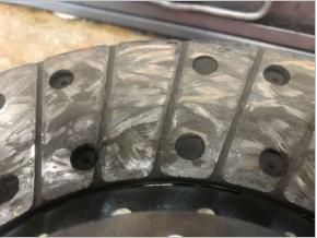
▲ Flywheel and Clutch Damage
