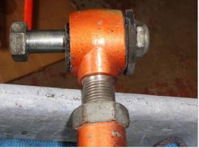
▲ All Control Arm Spacers and Bushings Damaged
