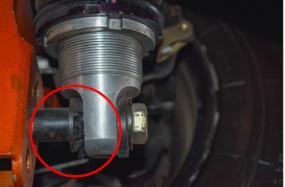
▲ ALL Coil Over Suspension Spacers and Bushings Damaged
