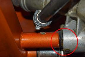
▲ Fluid Leaking from Rack and Pinion
